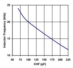
Figure 3: Typical Inductor Frequency vs. CHF Capacitor
