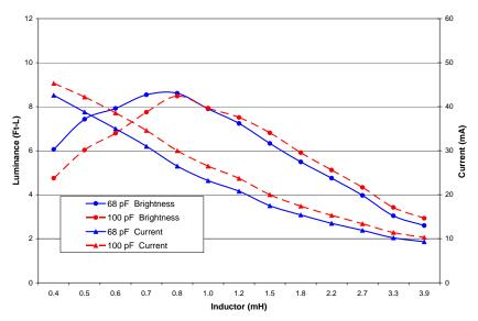
Figure 4: Luminance and current vs. inductor and CHF value. (Conditions: V+=3.0V, 2in<sup>2</sup> EL Lamp)
