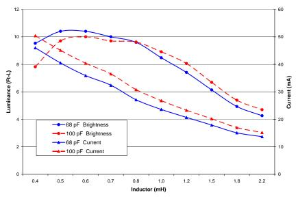
Figure 5: Luminance and current vs. inductor and CHF value. (Conditions: V+=5.0V, 4in<sup>2</sup> EL Lamp)
