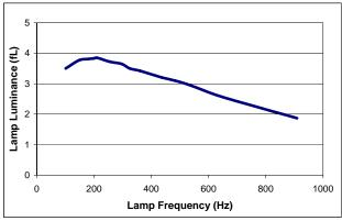
Figure 2: Luminance vs. Lamp Frequency (V+ = 3.0V, 2.4 in<sup>2</sup> DUREL 3 Green EL Lamp Load)
