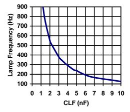
Figure 1: Typical Lamp Frequency vs. CLF Capacitor
