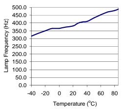
Output Frequency vs. Ambient Temperature
