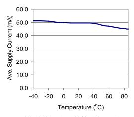
Supply Current vs. Ambient Temperature
