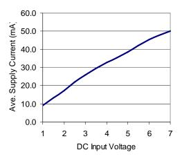
Supply Current vs. DC Supply Voltage
