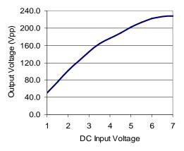
Output Voltage vs. DC Supply Voltage
