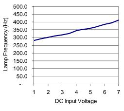
Output Frequency vs. DC Supply Voltage
