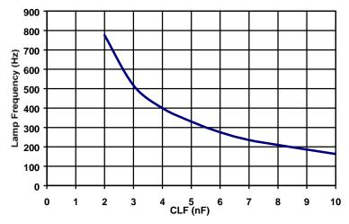
Figure 1: Typical Lamp Frequency vs. CLF Capacitor
