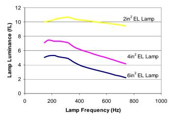
Figure 2: Typical Lamp Luminance vs. Lamp Frequency
