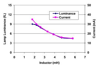
Figure 5: V+=5.0V, 4in<sup>2</sup> (25.8cm<sup>2</sup>) EL Lamp
