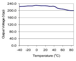
Output Voltage vs. Ambient Temperature
