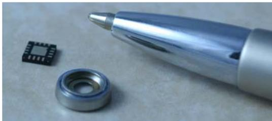
The D381 IC driver is also available as a "stand-alone" EL driver module solution that combines all required external discrete components, including a power inductor, into a small, 5mm X 7mm X 1.5mm lead-free (Pb-free) package. A D381 IC Driver Designer's Kit is available as a tool for optimizing the circuit for your application.
